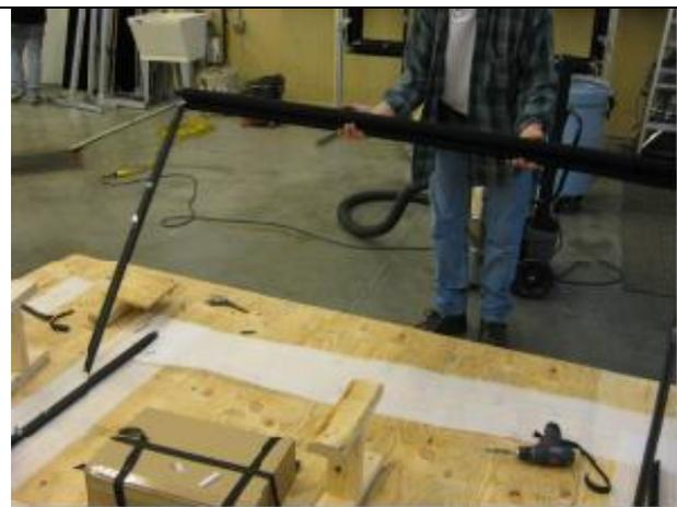
15) Remove the masking subframe from the crate and position the sections as shown previously with the main screen frame.
