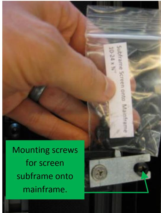
Mounting screws for screen subframe onto mainframe.
