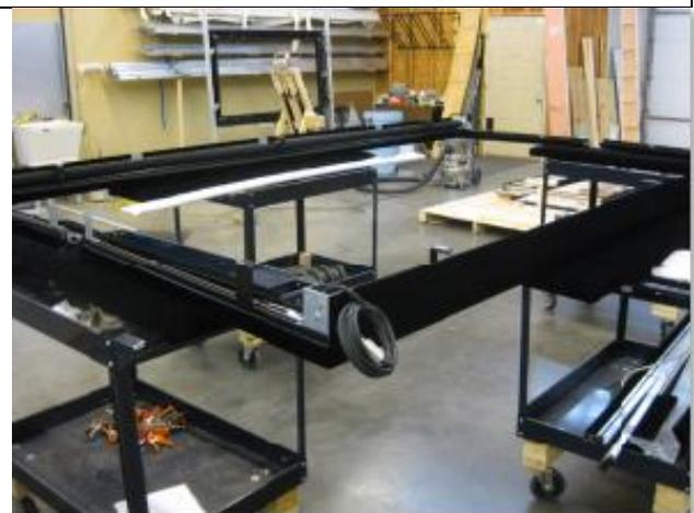
12) The main frame is now ready to be assembled using the splice bars provided.
