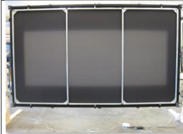
33) The photo above shows the back side of the projection screen assembly with the entire screen subframe installed.
