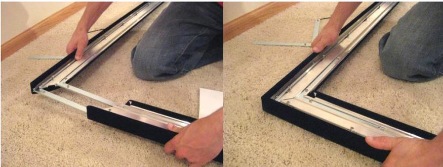
**Ball-Point Wrench the Set Screws.** Confirm with your fingers at the joint that they are perfectly joined and then start tightening the set screws. Use the ball-point end of the wrench provided so that you can more easily access the screws and won't over tighten them. Repeat this so that you've joined the top, bottom and one side piece, saving the other side piece for last.
