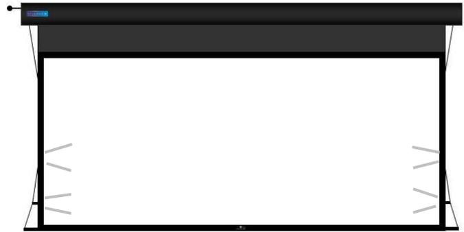
If you have “V” shaped wave patterns in the lower corners and/or fingering along the bottom, then your horizontal turnbuckles are too loose and need to be tightened. A couple signs that you've tightened them too much will be the opposite wave patterns (see below), or a slight separation of the screen material from the border velvet. This joint is very strong, but don't torque it to where you see visible strain or distortion of the screen shape.
