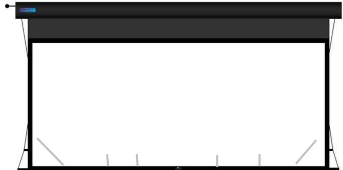
If you have the opposite pattern in the lower corners, then your horizontal turnbuckles are too tight and need to be loosened a bit. Generally, you want these tight to provide nice corner tension, but if you overdo it, not only will these patterns develop, but a visible gap will open between the screen and border material at the bottom corners. While the joint is strong, don't distort the screen geometry too much.
