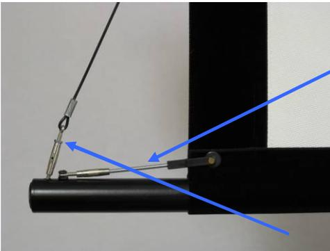
To adjust the tension, there are two turnbuckles on each side of the screen. The horizontal ones (hereafter called "horizontal") feature a standard thread on the rod joining the black plastic piece attached to the screen. Just focus your eyes on this half of the turnbuckle, so when we say "tighten," you think "righty-tighty, lefty-loosey." The other half with the screw is reverse thread and will mess with your mind.
