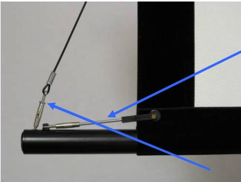
To adjust the tension, there are two turnbuckles on each side of the screen. The horizontal ones (hereafter called "horizontal") feature a standard thread on the rod joining the black plastic piece attached to the screen. Just focus your eyes on this half of the turnbuckle, so when we say "tighten," you think "righty-tighty, lefty-loosey." The other half with the screw is reverse thread and will mess with your mind.
