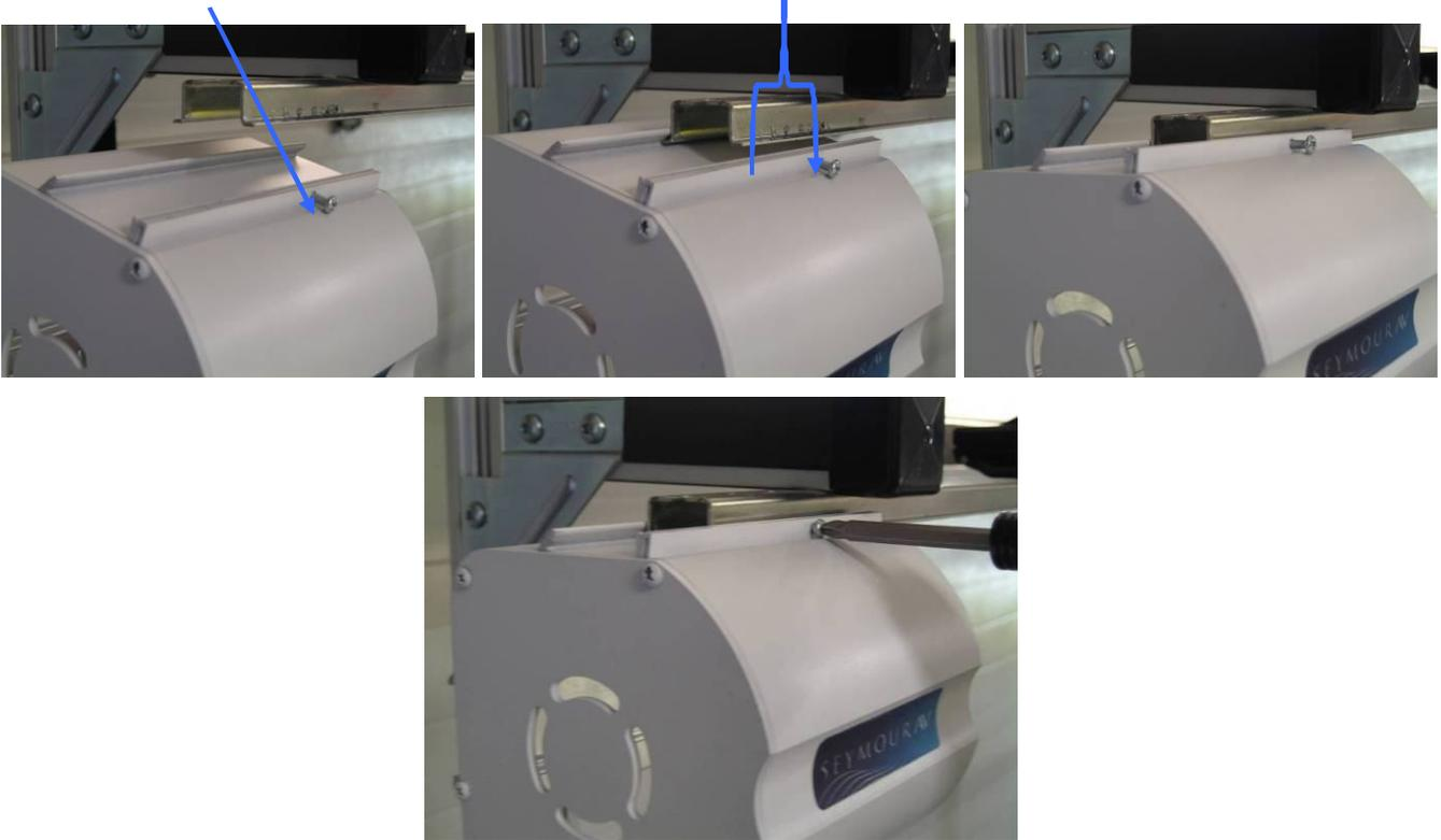
4) Approach the DIN rail with the screen case tilted down at a 30-40 degree angle. Your goal is to hook the extruded bevel into the back of the DIN rail fully. Once you have got that, you can then rotate the screen up to its resting spot and the DIN rail will nest inside that slot, just like it was when it was shipped to you. You must tighten at least one screw on each end so the case holds onto the rail.
