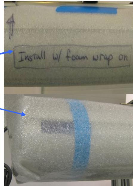
8) Note there are several pieces of tape and things that keep the materials where they should be. First, undo the blue Velcro straps you see on each end. These keep the weight bar happy during shipment, but **must** be taken off prior to operating the screen.
