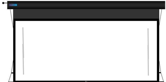
If you have horizontal wave patterns along the sides, then your vertical turnbuckles are too tight and they are lifting the bar. Loosen them up, and you'll find the ideal tension is where the bottom black tabs are snug to the cable but still easily slid up or down with your finger.
