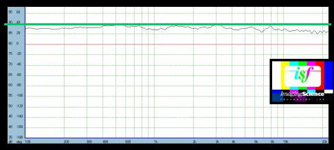
**Senlightor-Bright** The highest gain fine weave screen available anywhere. Gain 1.1, -1.5dB average attenuation, benign 20kHz roll-off.
