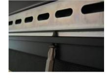
2) Locate the bag in the white remote box that has the five stainless steel truss head screws. Use a spirit level and mount the DIN rail to your wall using these screws. If you have a very curvy wall, you can
