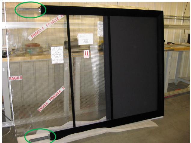
7. Lay the tall spacers (they have velvet on top, on top of a ~4" tall cardboard tube) where the center of the screen will sit, and the soft gray foam spacers (they have velvet on top, and are nicer than the white corner Styrofoam ones shown in the below pic) to cushion the outer edges. Do this again for the other side so you can lay both halves face down safely.
