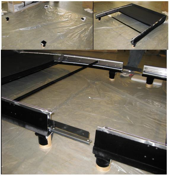
8. We kept the black velvet outer perimeter plates off of the top and bottom of the screen, so you can access the space where you bolt these center splice bars. Slide the halves together and align using the pins installed into the frame splice. In the accessories box, there is a bag of socket button head bolts for you to attach the four bars.
