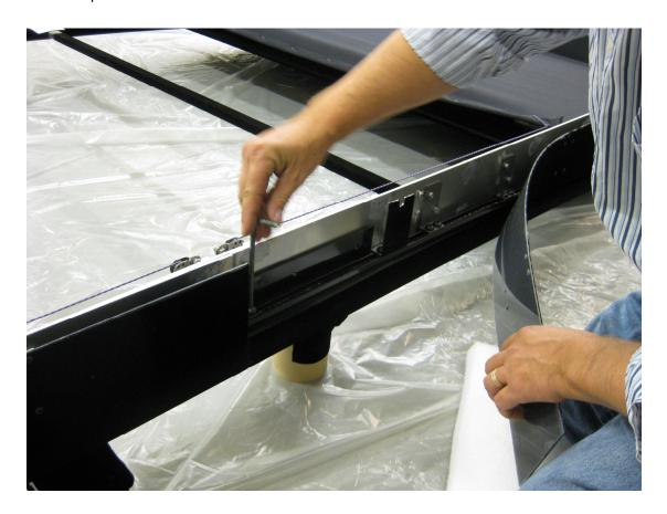
9. Hook up the masks as the picture shows. The (screen) left mask has red tape on it, along with the left mask card, indicating that it is the motor where we reversed the red and black power wires so that it acts opposite of the other mask. The motor power wires are installed into the terminal block either using the included white insertion key, or poking a screwdriver into the upper rectangular slot, depressing the spring that holds the wire.
